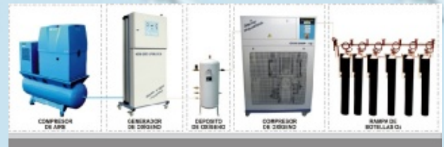
Schematic example For an oxygen cylinder filling plants
